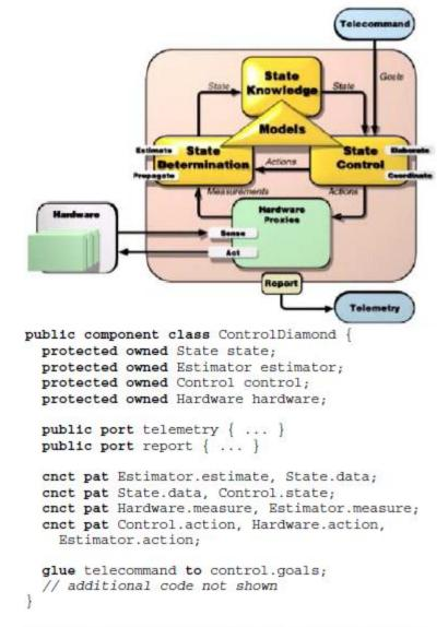
Figure 6. A graphical depiction of the Mission Data System architecture in use at the Jet Propulsion Laboratory, and simplified ArchJava code that captures the architecture.
