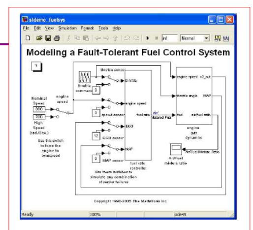
Figure 1: A Simulink model representing a controller. The basic blocks represent atomic mathematical operations like multiplications or differential equations. The model always shows the whole control behavior for a function, thus C code can be generated automatically, e.g. using dSPACE's TargetLink.
